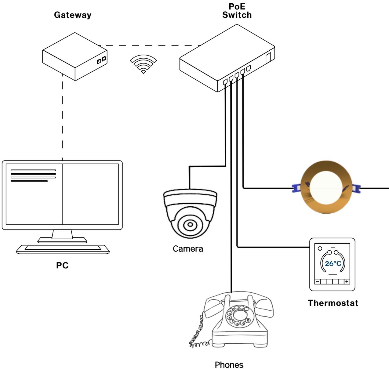
**PoE lighting** uses Power over Ethernet technology to connect, monitor, and control LED light fixtures used in smart building solutions. Smart PoE lighting reduces installation and operating costs by more than half and helps building owners meet wellness and sustainability goals. Since the low voltage PoE system does not require shielded cables, conduit runs are eliminated early in the construction process.
