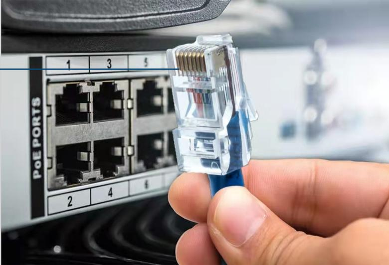
Power over Ethernet ( PoE ) is a standard for passing electrical power and data through a network cable, thus eliminating the need for a separate power supply and AC outlet to power connected devices.
