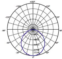
BL4-FM55-30K CCT:3000K LEDs input watts: 10.5W delivered lumens: 721, LM/W = 68.94 test no. LCZP22060184 tested in accordance to LC-I-902 GMS-2000
