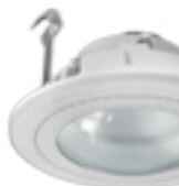
B35602 3.5" Shower Trim with Dome Lens Lamp: MR16 LED GU5.3 6W Max. GU10 LED GU10 6W Max. PAR16 LED E26 6W Max. Gasket used to prevent moisture Wet location listed
